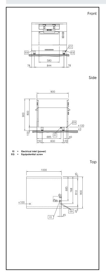
Modular Cooking Range Line thermaline 90 - 4 Zone Electric Solid Top on Oven, 2 Side H=800
